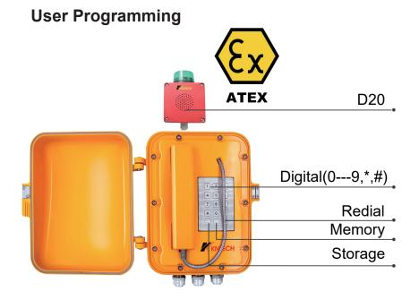
pick up the Handset, press the keyboard storage key+address key (digital 0 --- 9) +phone number+storage key, and then hang up.
