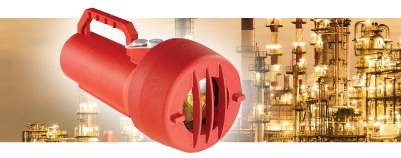
The General Monitors TL105 is a battery operated, rechargeable test lamp specifically designed to test General Monitors' UV, UV/IR and IR flame detectors. The test lamp provides a high-energy, broadband radiation source that emits sufficient energy in both the ultraviolet and infrared spectra to activate UV and/or IR flame detectors. To simulate a fire, the test lamp automatically flashes at various selectable rates.
